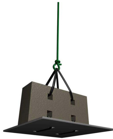
Figure 8. A SETL-plate and deployment of SETL-plates in the Wash estuary UK.
